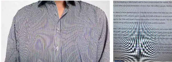
Figure 1: Moire fringes produced by the interference between the camera's pixel grid and a periodic subject: a striped shirt (left, from [1]) and a computer monitor (right, from [2]).
